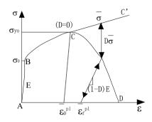
Fig. 3. Stress-strain curve with progressive damage degradation
