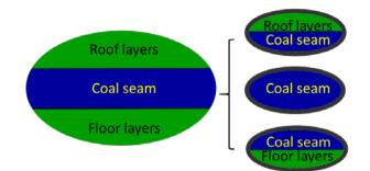
Fig. 4. Three working conditions of cutting head
