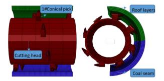
Fig. 5. The model of cutting roof-coal layers
