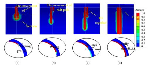
Fig. 6. Crushing process of coal-rock
