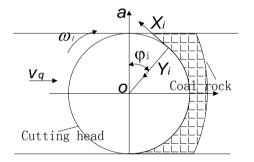
Fig. 2. Mechanical model of bolter miner cutting head
