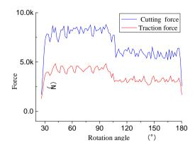
Fig. 8. Force curve of a pick cutting roof and coal
