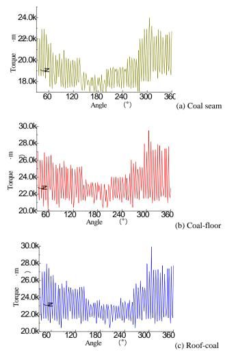
Fig. 11. Torque variation curve of cutting head
